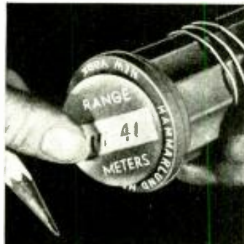
Above: Inserting the "range" disc, after the wavelengths have been properly written in. Right: the large openings in the pins, where the coil winding leads enter and are soldered.
