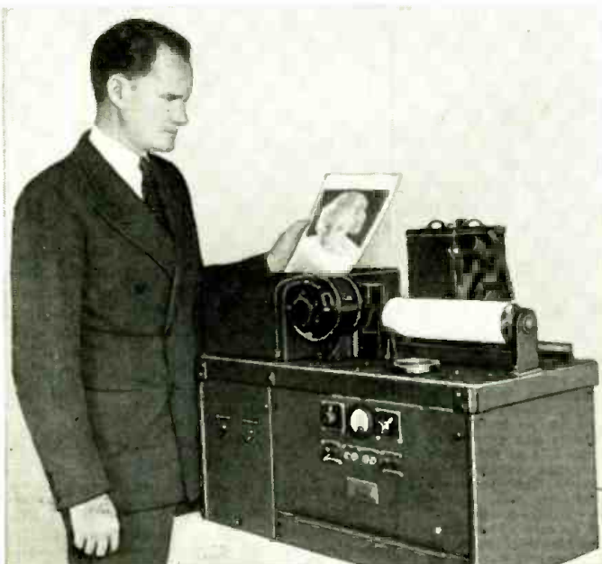
Photos, maps and complete telegraph messages can now be successfully transmitted and received at high speed, by means of the new facsimile recorder here shown.
